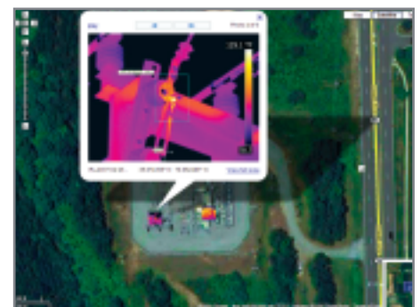
P660's embedded GPS tags your IR images so you can zoom in on exact locations and speed repairs.
